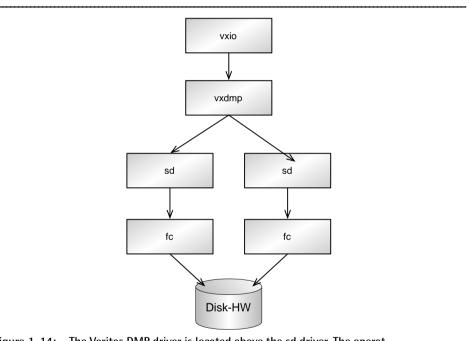
Figure 1-14: The Veritas DMP driver is located above the sd driver. The operating system offers the DMP driver several paths to each disk
