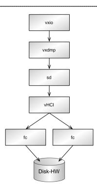
Figure 1-13: The Sun vHCl driver is located below the sd driver. The operating system only offers the DMP driver a single path to each disk
