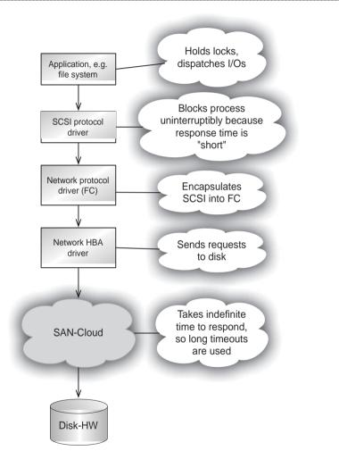
Figure 1-19: Layered device drivers become a big problem if the upper layers expect a rapid response, but the lower layers do not deliver as rapidly. Locks, memory, and process contexts get stuck for an extended time, eventually leading to deadlock situations.
