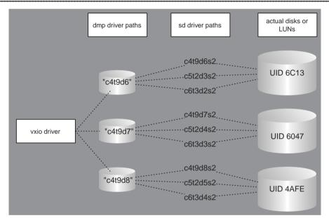
Figure 1-15: Upon initialization, DMP reads all the SCSI disk device nodes and finds their universal ID. It maps all nodes that return the same UID to a logical device and gives it a unique "access name". Subsequently, accesses to that UID are routed over all available paths that originally returned the same UID. The standard sd driver remains functional, but is unaware of the fact that many of its paths are actually the same device.
