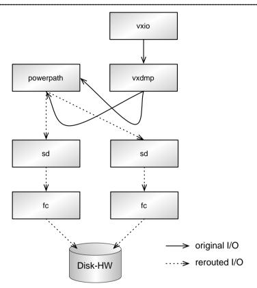
Figure 1-16: The EMC powerpath driver is located at the same level as the DMP driver. The operating system offers the DMP driver several paths to each disk, but usage of these paths is caught and redirected by powerpath
