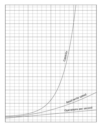
Figure 1-1: Non-quantitative graph showing how Moore's law only applies to disk capacity, while bandwidth and particularly operations per second are left behind. The X axis shows the years, while the Y axis shows the criterion that the curves are labelled with. Note that for the most importance today, namely TX/sec/GB, the capacity (which grows exponentially) is in the denominator, leading to exceedingly poor random read performance!
