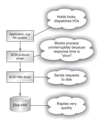
Figure 1-18: Drivers for devices which are considered to respond quickly will allocate resources much more aggressively, since the response is due in very short order anyway. The I/O is made uninterruptible for performance and other reasons.
