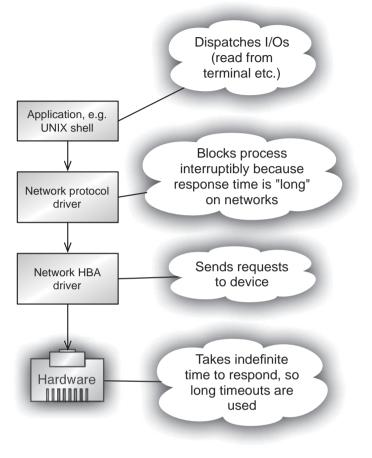
Figure 1-17: Drivers for devices which are known to exhibit potentially slow response times sleep interruptibly. They also typically do not require a lot of resources, and the applications that use them will not keep important data structures locked while they do I/O.
